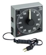
**Automatic Enlarger Timing** Plug enlarger into outlet marked ENLARGER. Set TIME-FOCUS switch to "focus". Turn ON-OFF switch to "on" and focus enlarger. Then turn to "off" again. Set timer hands clockwise to desired setting. Also, set TIME-FOCUS switch to "time". Turn ON-OFF switch to "on". Desult: Timer will outper witch the set of the replaced time interval. Result: Timer will automatically turn enlarger off after selected time interval. Description ltem# MCRD
